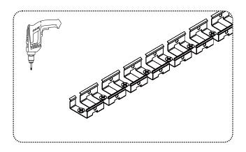
I. Fix the moldable groove with screw
