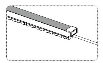
2. Insert the strip into moldable groove
